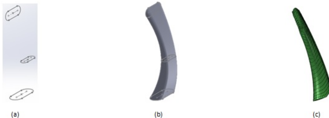
Figure 6.4: a) Sketch of ACL cross-sectional areas b) ACL after loft feature c) ACL in ABAQUS
